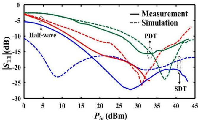
Fig. 2 Measured and simulated  $|S_{11}|$  of SDT and PDT rectifiers versus  $P_{in}$ .
