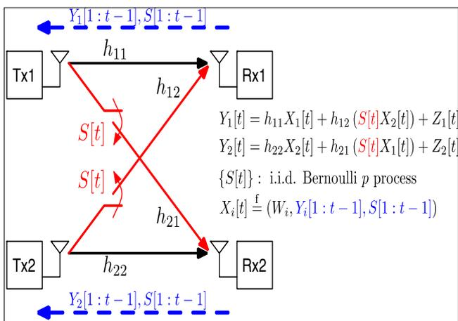
Figure 1. Two-user bursty interference channel
