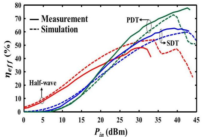
Fig. 3 Measured and simulated  $\eta_{eff}$  of SDT and PDT rectifiers versus  $P_{in}$ .
