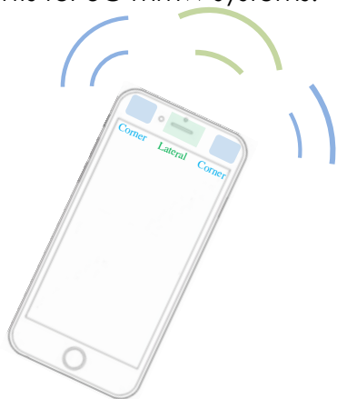
Fig 1. Placement of the end-fire antennas in a mobile terminal with the corner and the lateral designs.
