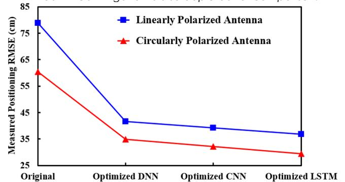
Fig. 4. Measured positioning RMSEs of tag locations with various optimized models using the linearly polarized antenna and the proposed circularly polarized antenna. The original measurement result without NLOS mitigation is also depicted for comparison.
