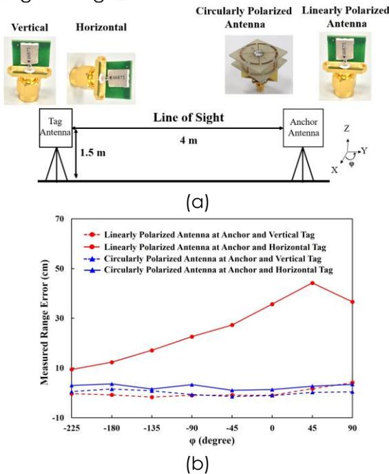
Fig. 1. (a) Measurement setup of one-to-one ranging system. (b) Range errors measured by one-to-one system with the linearly polarized antenna and the proposed circularly polarized antenna.
