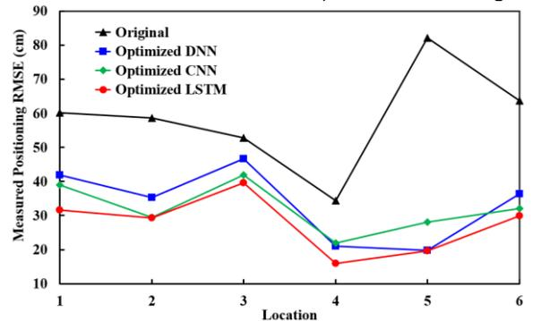
Fig. 3. Measured positioning RMSEs of tag location 1 to 6 with various optimized models. The original measurement result without NLOS mitigation is also depicted for comparison.
