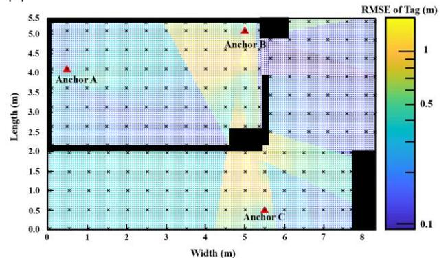
Fig. 2. Floor plane for UWB positioning system verification. The 226 candidate anchor locations are shown as the crosses, and the simulated RMSEs of all tag locations with best anchor placement are depicted as the colored squares. The values of RMSEs are shown in log scale on the right-hand side, and the three best anchor locations are depicted as red triangles.
