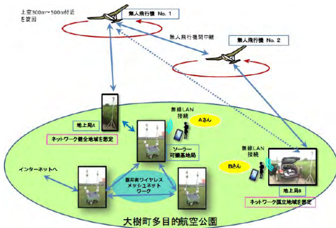
Figure 5. The UAV-utilized technology to relay wireless signals for online connection with the disaster-stricken area. Image source: NICT News, URL: https://www.nict.go.jp/press/2013/07/17-1.html
